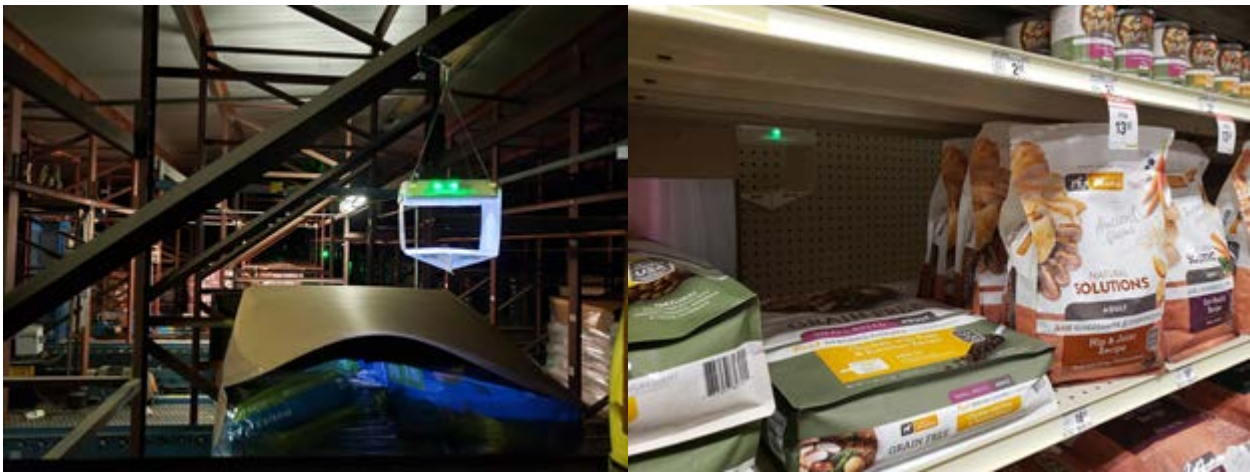
Left: SightTrap installed at a retail pet food store to help protect products and brand names from stored product insects. Right: SightTrap installed at a fully automated warehouse where individuals are unable to access hard to reach areas to monitor for stored product insects on a routine basis.
