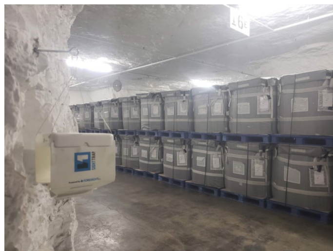
A SightTrap remote pheromone monitor is hung near to seed storage in a cave.
